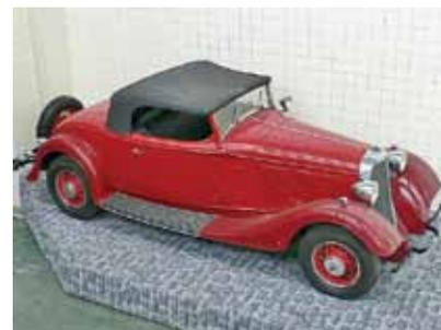
■ Dammann & Wagner tell us, in *The Cars of Lincoln Mercury*, that this 1933 Lincoln is Model 520-A with trunk deck. At a cost of \$2,900, it weighed about 4,750 lbs. and had a lined top. This was the first year for the new smaller V-12 engine of 381.7 cubic inches and 125 horsepower. The KA-1029 serial number was near the end of the run.
